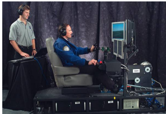
Figure 1.—Ice contamination effects flight training device.
