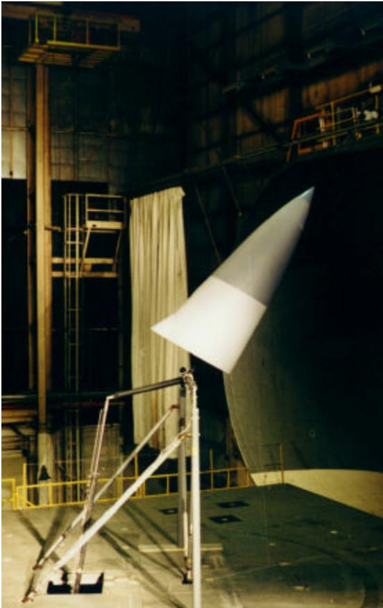
Figure 1 F-15 Radome in the Langley 30x60 Full Scale Test Section.
