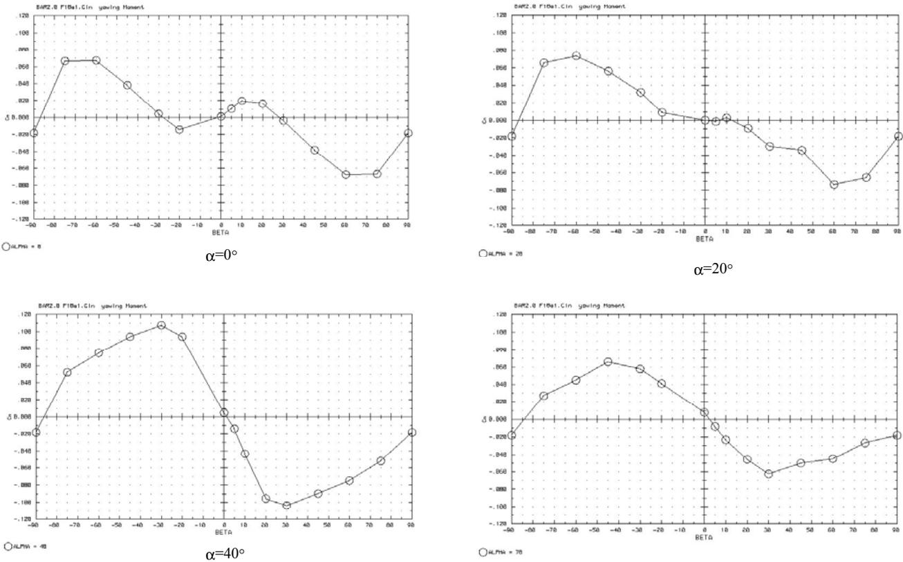
Figure 9. Effect of Sideslip on Yawing Moment
