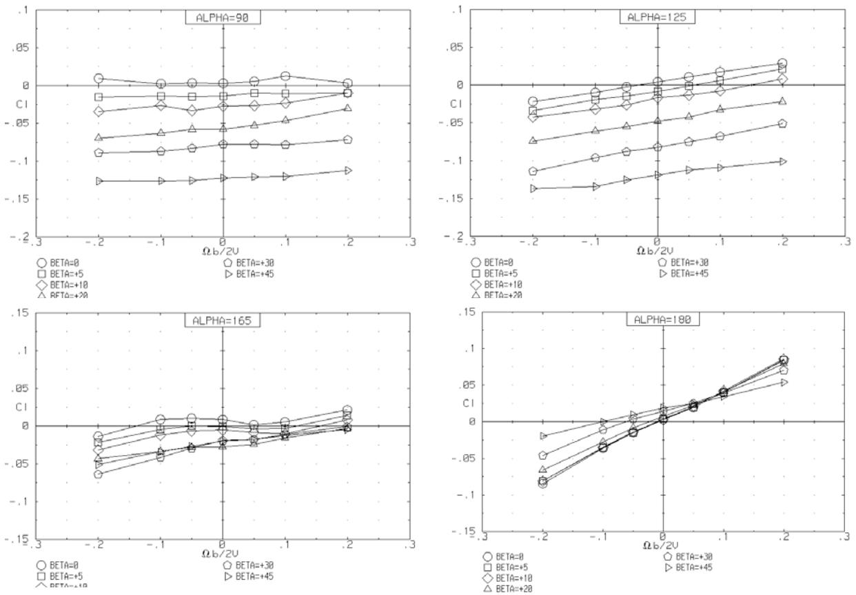
Figure 8. Large-Angle Rotational Rolling-Moment Characteristics
