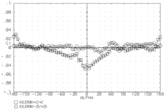
Figure 7. Effect of Aileron Deflection at Large Angles of Attack
