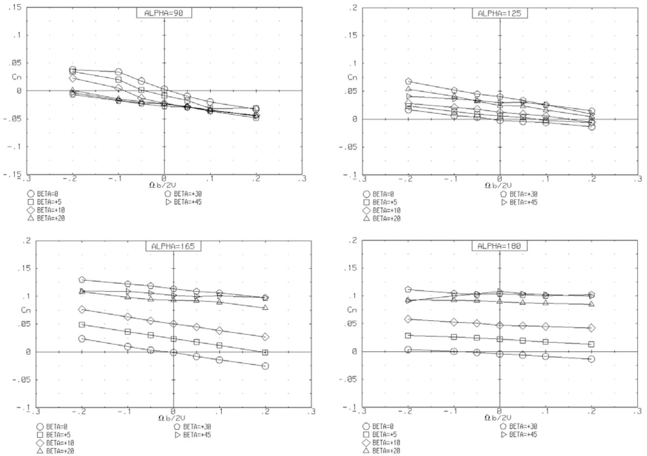
Figure 11. Large-Angle Rotational Yawing-Moment Characteristics
