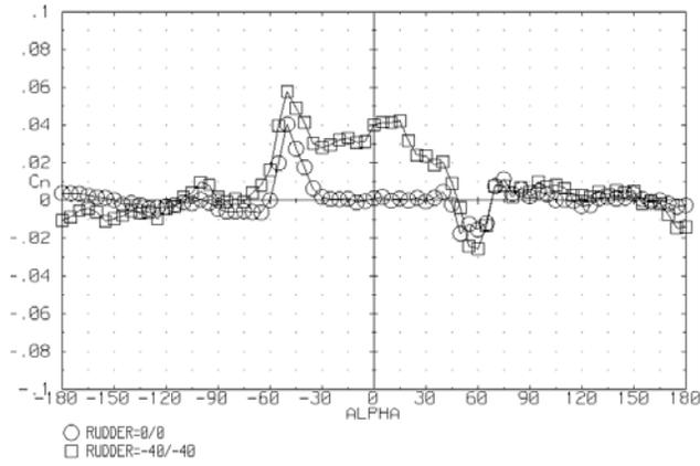
Figure 10. Effect of Rudder Deflection at Large Angles of Attack
