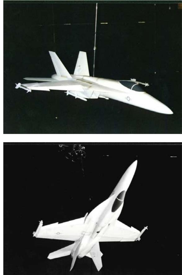
Figure 1. Large-Angle Testing of the F/A-18E/F Model.
