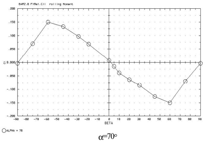
Figure 6. Effect of Sideslip on Rolling Moment
