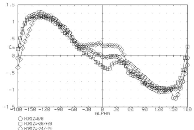
Figure 3. Effect of Angle of Attack and Horizontal Deflection on Pitching Moment
