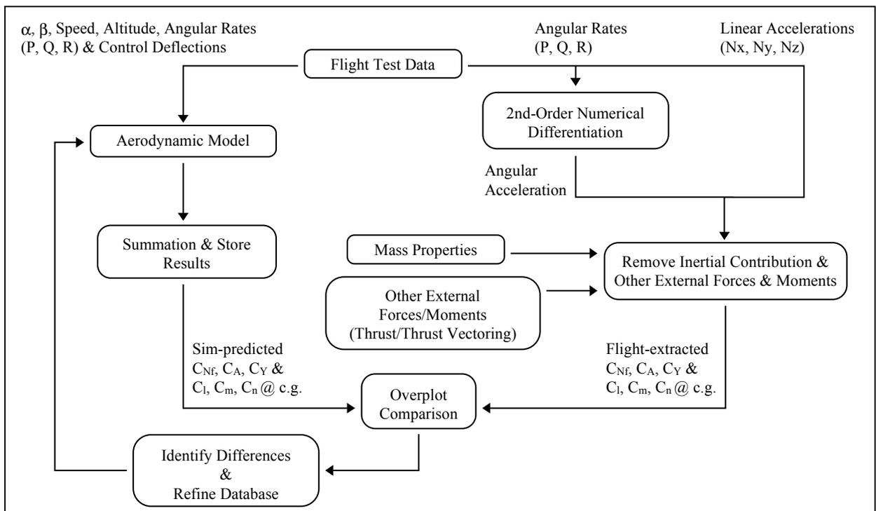
Figure 13. Schematic Of Typical 'OverDrive Technique.
