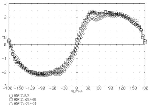
Figure 2. Effect of Angle of Attack and Horizontal Deflection on Normal Force
