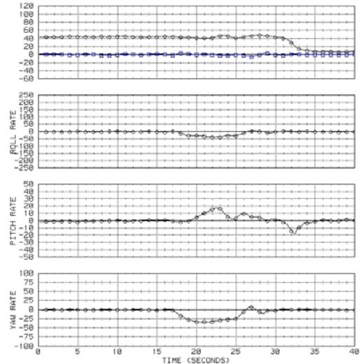
Figure 3a. Velocity vector roll rates and angles
