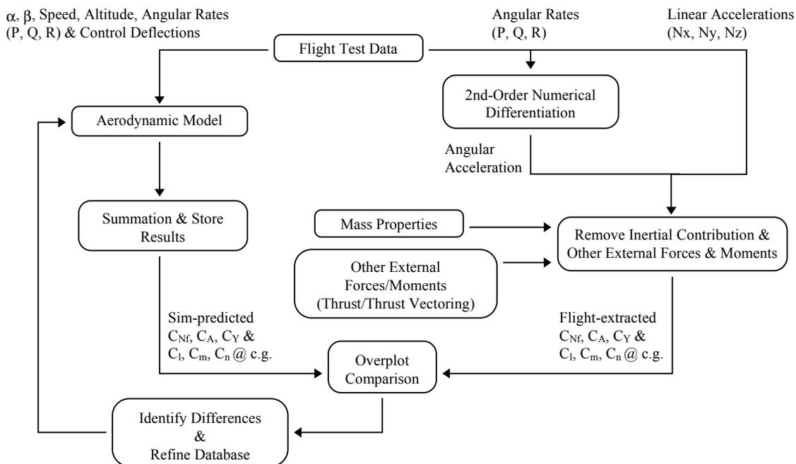
Figure 2. Schematic of 'Overdrive' technique
