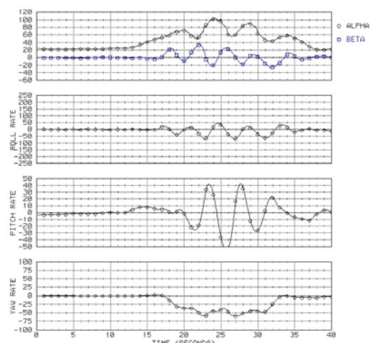
Figure 6. High aoa spin motion, rates and angles
