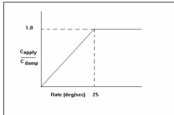
**Figure 3.** Schedule for Applying Damping Moments During Simulations
