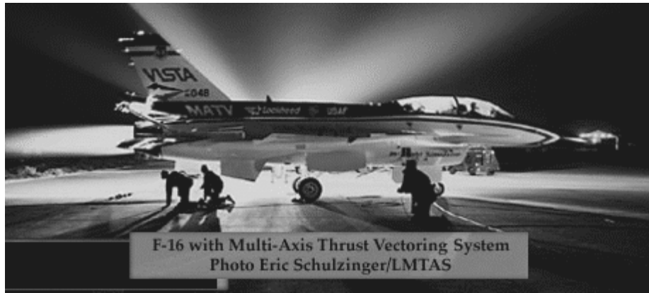
Figure 1.- Variable-Stability In-Flight Simulator Test Aircraft with Multi-Axis Thrust Vectoring.
