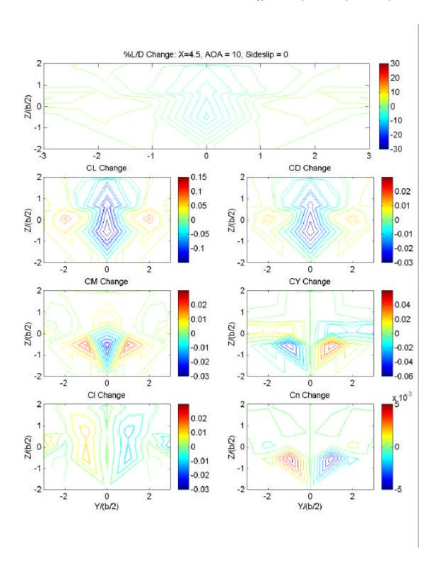
Figure 6. Aerodynamic effects on the test configuration at X position 4.5b/s,  $\alpha = 10^{\circ}$  and  $\beta = 0^{\circ}$  resulting from formation position.
