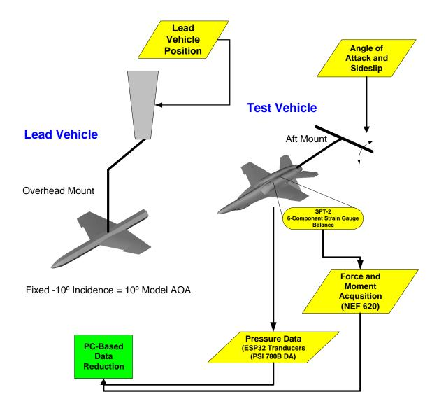
Figure 2. Diagram of test apparatus and set up.
