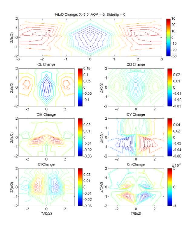
Figure 3. Aerodynamic effects on the test configuration at X position 3.0b/s,  $\alpha = 5^{\circ}$  and  $\beta = 0^{\circ}$  resulting from formation position.
