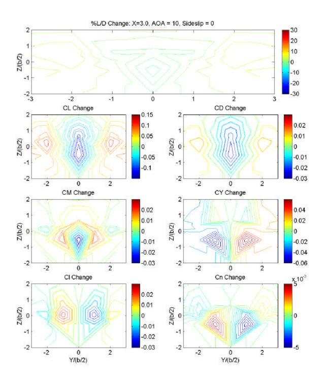
Figure 4. Aerodynamic effects on the test configuration at X position 3.0b/s,  $\alpha = 10^{\circ}$  and  $\beta = 0^{\circ}$  resulting from formation position.
