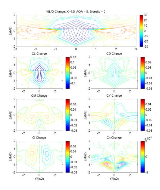
Figure 5. Aerodynamic effects on the test configuration at X position 4.5b/s,  $\alpha = 5^{\circ}$  and  $\beta = 0^{\circ}$  resulting from formation position.
