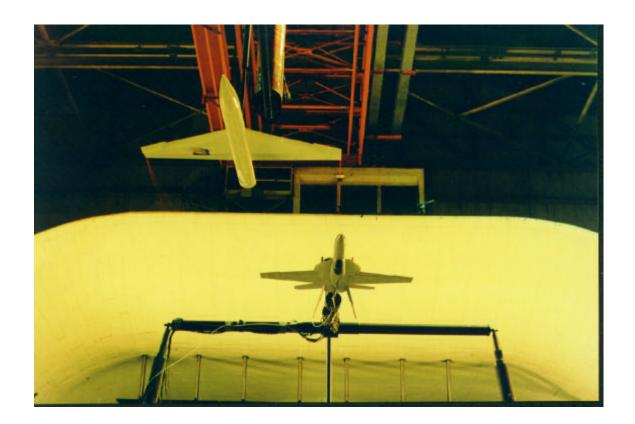
Figure 1. Photograph of a two aircraft formation in the Langley Full-Scale Tunnel.
