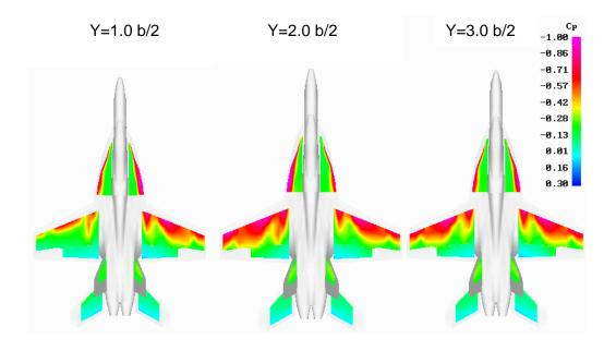
Figure 7. Top-surface pressure distribution of the test aircraft at  $\alpha=5^{\circ}$  and  $\beta=0^{\circ}$  for three span-wise formation positions.
