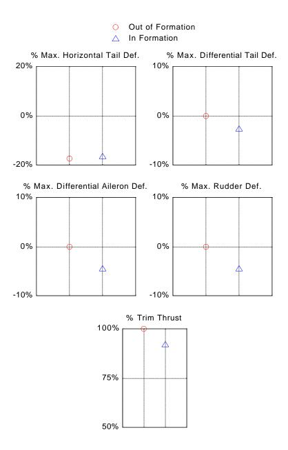
Figure 8. Trim control requirements for close formation flight.
