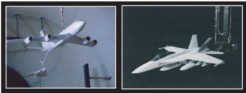
Bihrlle Applied Research Inc leads the industry in advanced wind tunnel test techniques designed to collect aerodynamic data throughout the flight envelope.
