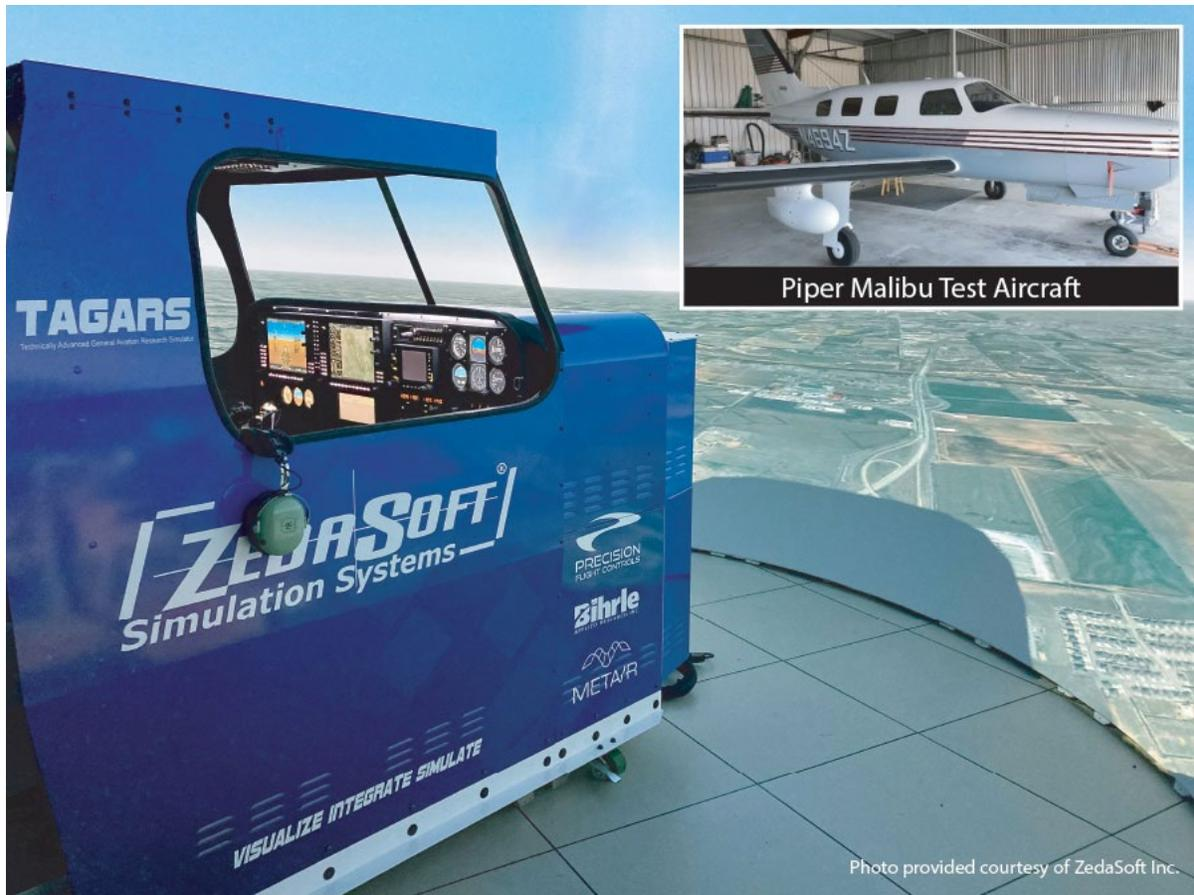
*Image: Technically Advanced General Aviation Research Simulator (TAGARS) with inset photo of Malibu flight test aircraft (Background image courtesy of ZedaSoft).*
